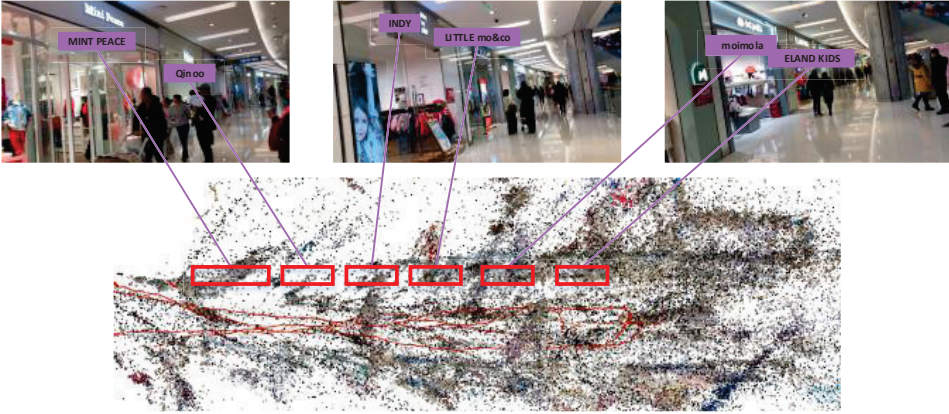
Fig. 4. An illustration of the text localization method. The bottom figure represents the sparse point clouds of the part of the indoor scene generated by the colmap algorithm. The red rectangles in the point clouds represent the text locations extracted from the top three images in the indoor scene.
